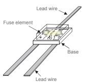
When the ambient temperature rises to the operating temperature of the D6-type, the fuse element melts, and forms a drop around the end of each lead because of surface tension and the special flux coating. This cuts off the electrical circuit. In another scenario, the heater resistance generates heat in response to an external signal, thereby melting the fuse element and cutting off the electrical circuit immediately.
